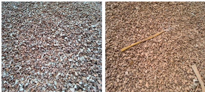
Figure 7 Image of iron ore lumps washed with only water and water and dispersant together
