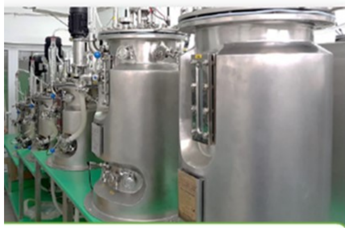
Figure 11 Integrated bioleach Pilot plant facility, capacity 20L pulp/day
