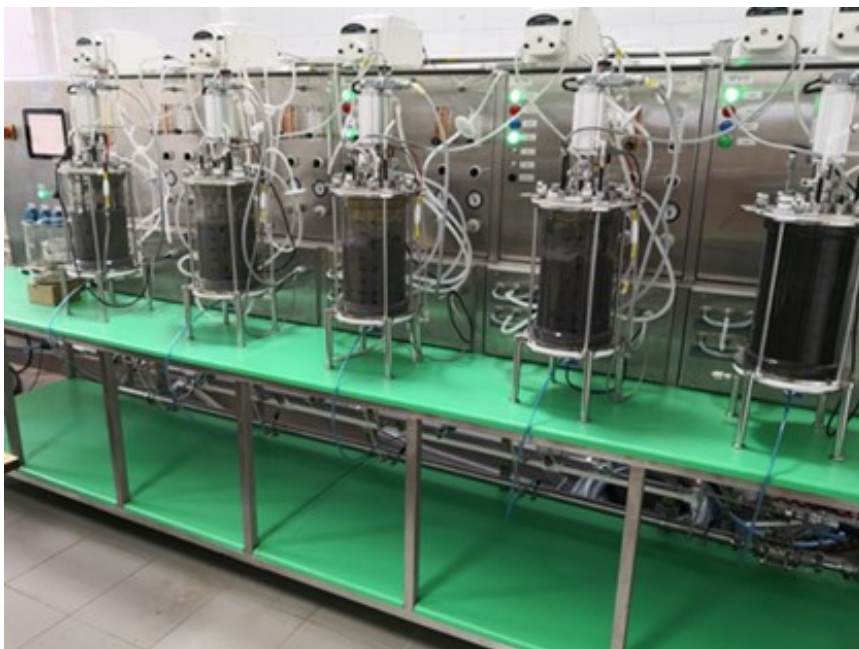
Figure 10 Small scale continuous bioleach reactors of ore with a capacity of 1L pulp/day
