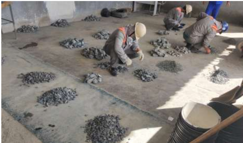
Figure 2 Hand-sorting in FERBASA. Rocks are manually classified according to their lithology and size
