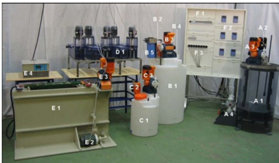
Figure 13 Laboratory plant for leaching, solvent extraction and electrowinning A1 - reactor for leaching, B1 - feed tank for bioleach solution, C1 - tank for organic solution, D1 - mixer - settlers, E1 – electrowinning cell, F1 - control panel
