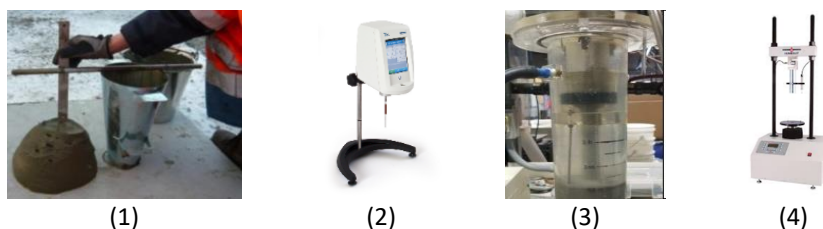
Figure 1 12" (300mm) ASTM Cone (1), Brookfield Device (2); Thickening Test (3) and Backfill Strength Testing Machine Apparatus
