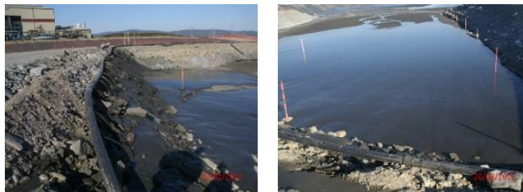
Figure 5 Paste Deposition in Thin Layers for High Sulphide Tailings (MATSA mine)
